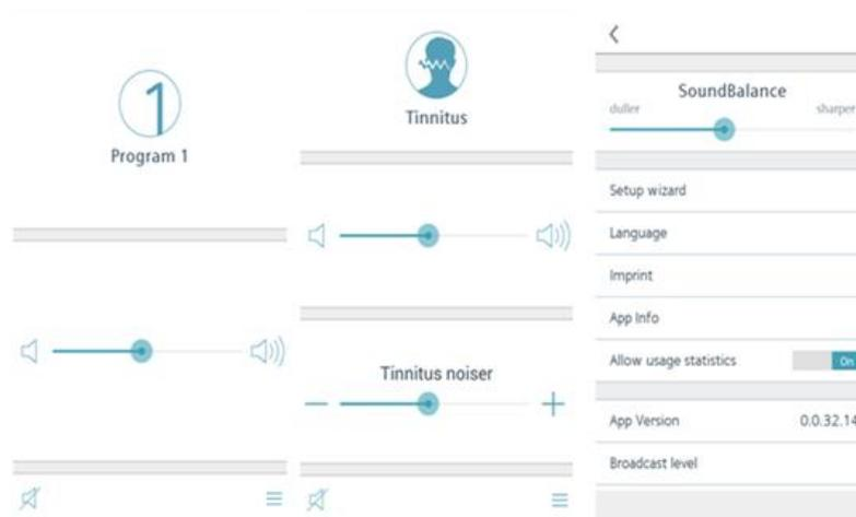
Figure 5: Program change, volume control, tinnitus control and sound balance remote control functions provided by the touchControl App on a smart phone.
