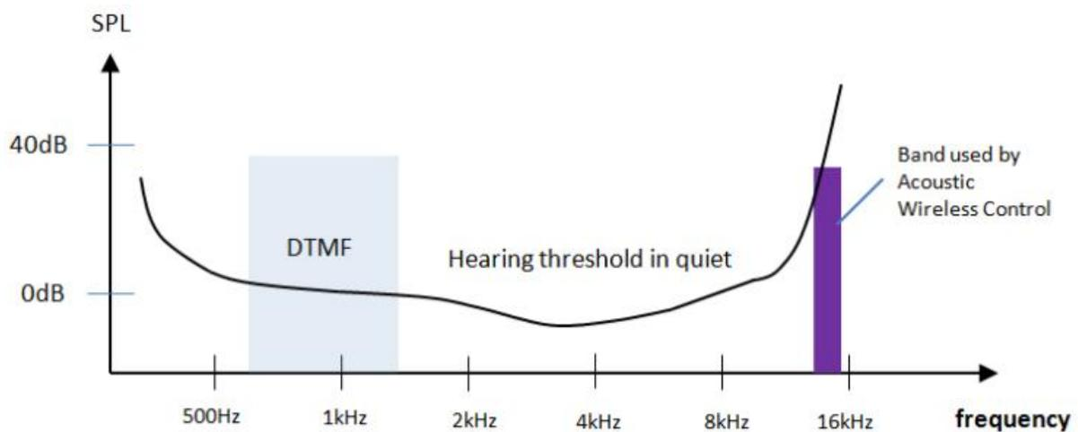
Figure 2: Frequency band used by the Acoustic Wireless Control compared to a hearing threshold in quiet.
